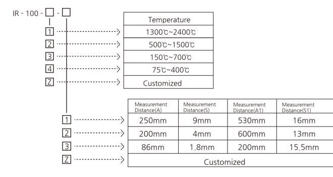
For example "IR-100-1-1" indicates 1300°C~2400°C temperature, 250mm measurement distance(A), 9mm measurement distance(S), 530mm measurement distance (A1) and 16mm measurement distance(S1).
