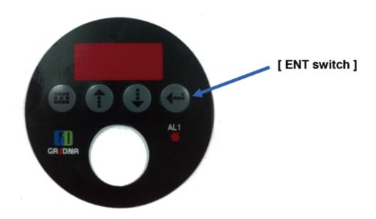
To aim a target object, enter the switch. Please press ENT switch for laser pointer on/off.
