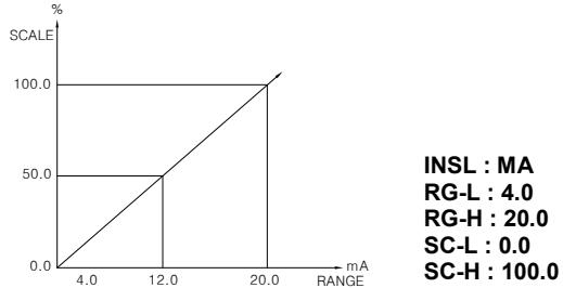
4.2.1 According to this program, DI-20 automatically calculates the input signal values into displaying scale values.
