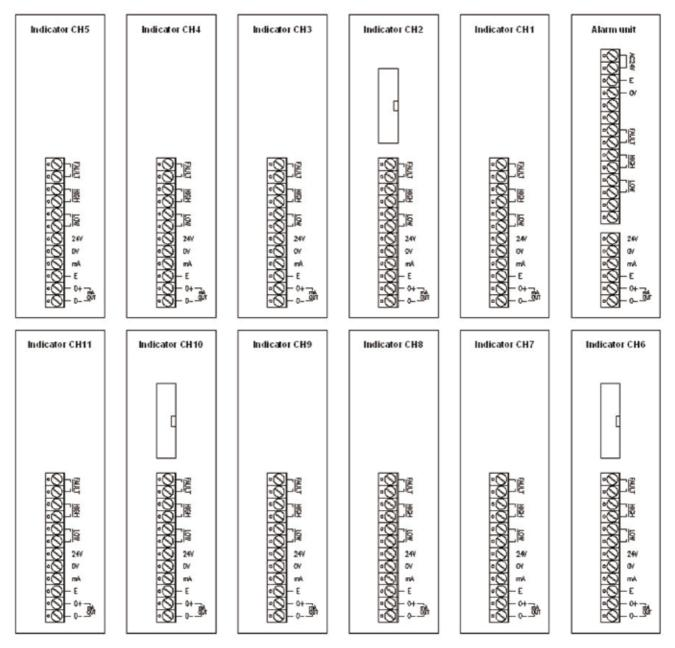
Note: Every channel has two terminals each of FAULT, HIGH, & LOW.
