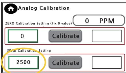
After connecting the standard gas for SPAN calibration, enter the concentration of the standard gas in the yellow circle and press Enter.
