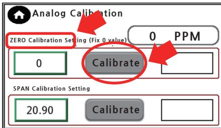
Connect the nitrogen gas and set the ZERO calibration.
